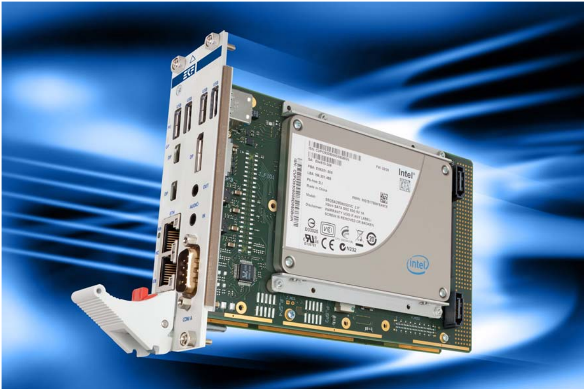
PC4-PRESTO w. PCS-BALLET Side Card & 2.5-Inch SSD, 8HP
